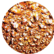
Varnish on reservoir ceiling (Stalactites)
