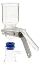
Glass filter funnel + filter holder top assembly
