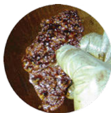
Varnish can be hard and brittle (Lacquer)
