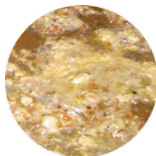
Varnish deposits on reservoir floor (Plated)
